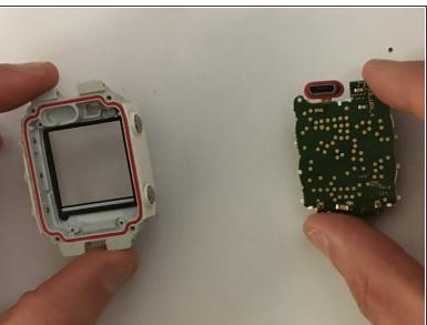
Detach the screen from the screen protector using a PH000 screwdriver.
