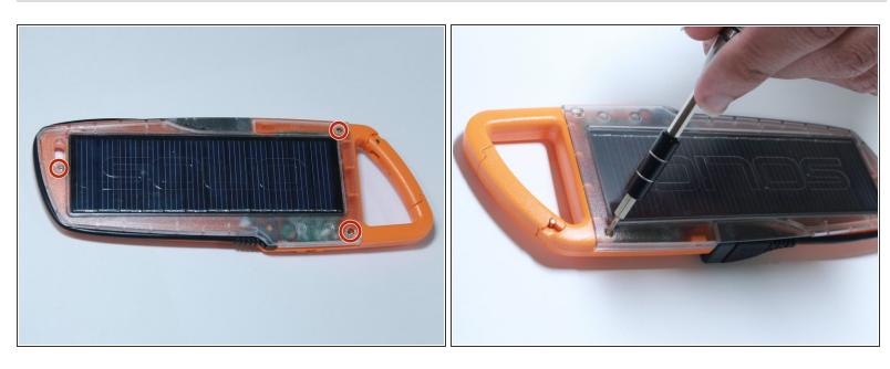
Locate, and unscrew, the three 5.72 mm screws that hold down the top cover using the T6 Torx screwdriver.
