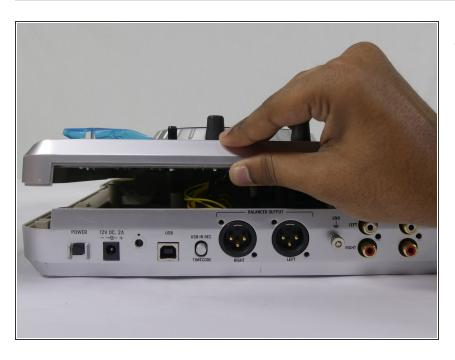
Using your fingers, gently pull apart the two panels of the device until you feel resistance from the cables.
