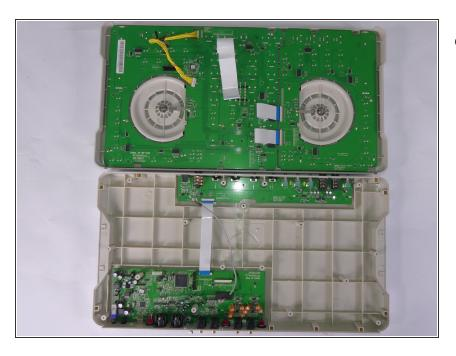
Open the two panels completely, gently placing each side on your working area to avoid damage to the buttons on the outside face.
