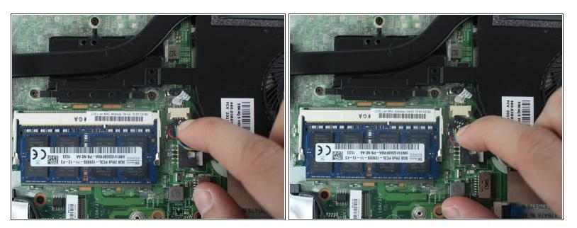
• Unplug the Fan connector from its socket on the motherboard.
