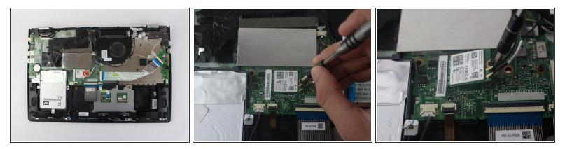
• Remove the 5.4 mm Phillips #0 screw holding the Wireless Network Card.
