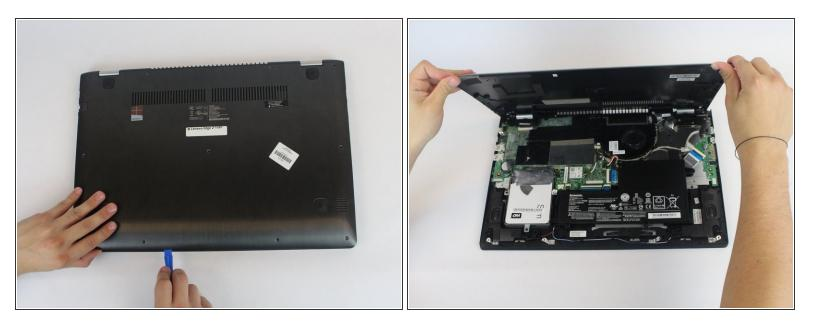
Using a plastic opening tool, pull out the back panel from the laptop.
