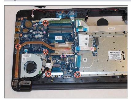
Unscrew the five screws securing the motherboards.
