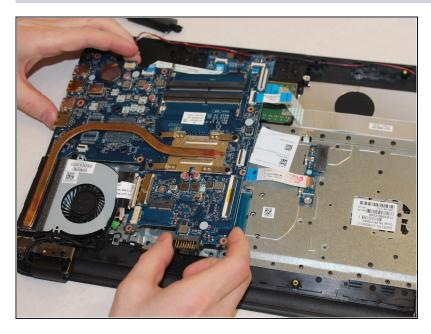
Gently lift the motherboard up and out of the casing.
