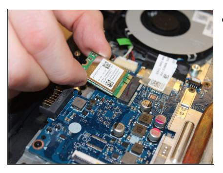
carefully pull the card of its slot.
