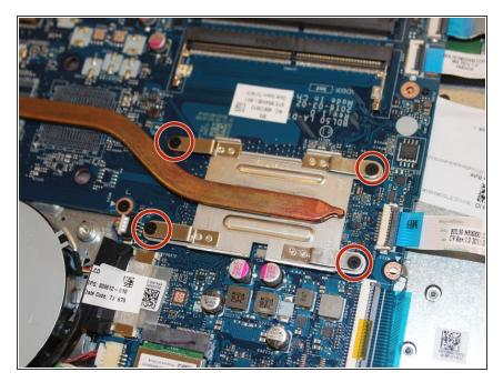
Remove the four screws holding the heatsink on.
