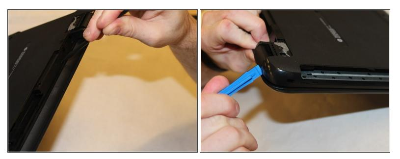
Using the spudger, push in the tabs in the back that hold the body together. Carefully pry the body apart by working the spudger around the body.
