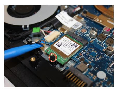
Using the size #00 Phillips screwdriver remove the single screw holding it in place.
