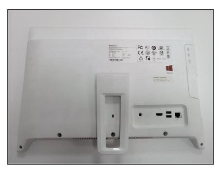
Turn the PC around, and get out the 5 screws from the bottom
