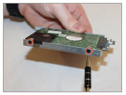
Remove the 4 screws holding the hard drive to the hard drive cage using the Philips #00 screwdriver.
