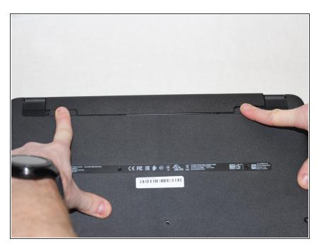
With the device turned upside down, use your index fingers to push the battery latches in towards each other.
