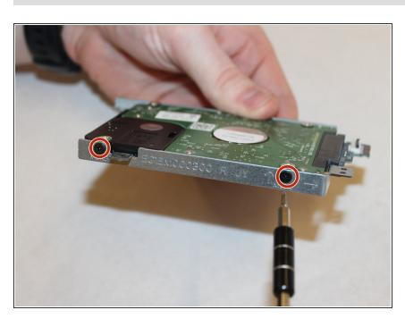
Remove the 4 screws holding the hard drive to the hard drive cage using the Philips #00 screwdriver. To reassemble your device, follow these instructions in reverse order.
