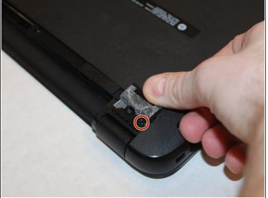
Remove the highlighted screws holding the body of the laptop together with a size #00 Phillips screwdriver.
