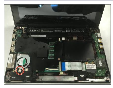
• Unclip the connector that is located above touch screen
