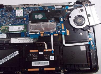
Next, carefully remove the sliding connector that connect the CPU Fan and the laptop together using the tweezers.
