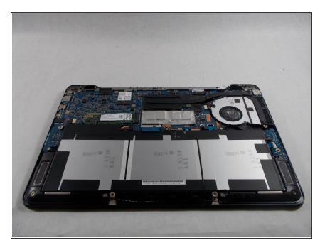
Locate the battery near the bottom.
