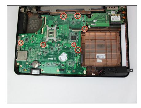
Unscrew the indicated 5.6mm screws with a Phillips #0 screwdriver.
