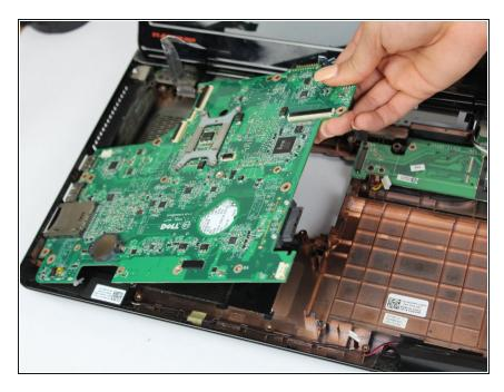
• The motherboard can now be removed by pulling upwards, tilting it to the left of the laptop until the connectors clear the body of the laptop.
