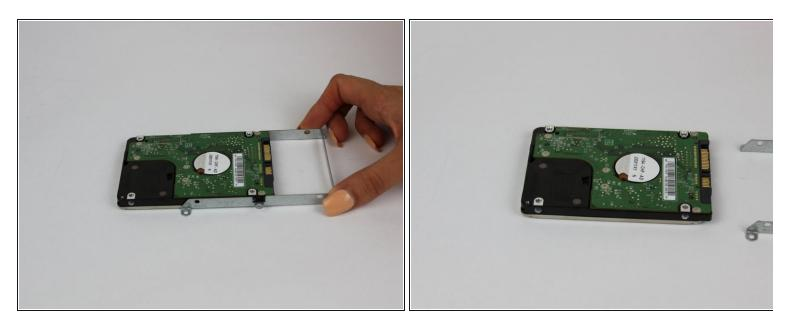
• Slide the assembly off of the hard drive.
