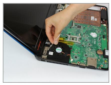
• Remove the fan from the device.
