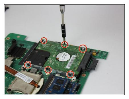
Unscrew the 6 Phillips head screws holding the hard drive to the motherboard with the #0 driver head.
