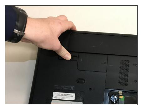
In the top left corner, there is a lever that has a small picture of a battery on it. Slide the lever to the left.
