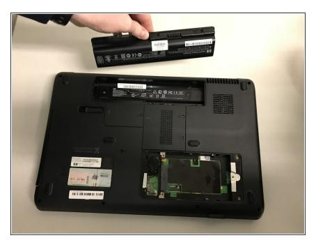
The battery can then be pulled out of its compartment by hand.
