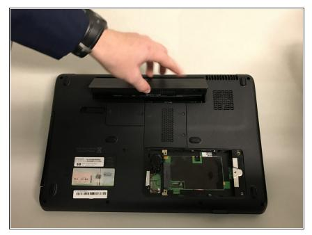
Once you have slid the lever to the left, the front part of the battery will be released and you should be able to grab the released part of the battery with your thumb.
