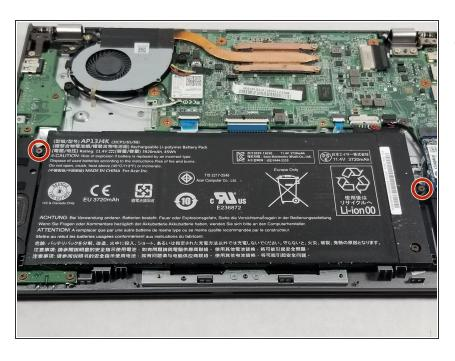
Unscrew the two 5mm battery screws using the Phillips #0 screwdriver.
