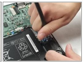
Remove the 3.75 mm screw with a Phillips #0 screwdriver.
