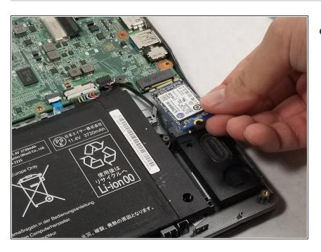
Pull the Solid State Drive out of the connector.
