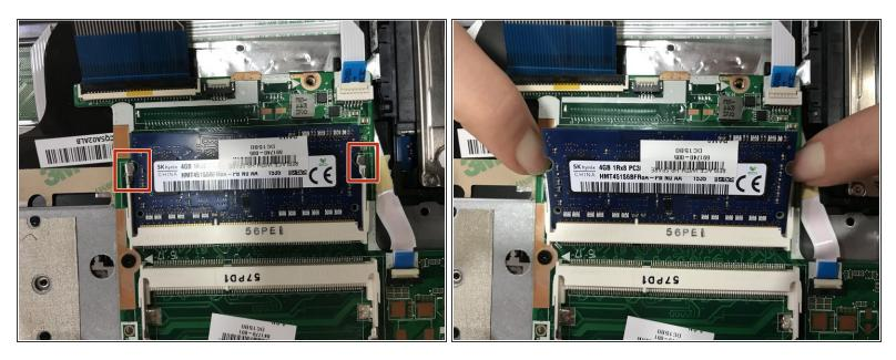
• Release the RAM by pulling the two white levers away from the sides of the RAM.
