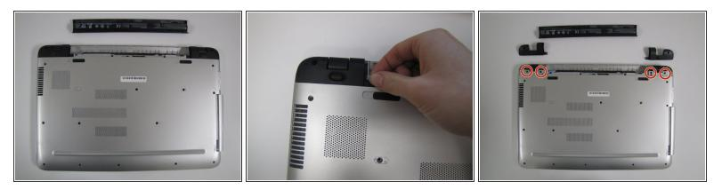
Remove the black corner covers on either side of the battery to reveal four additional 6.5mm
