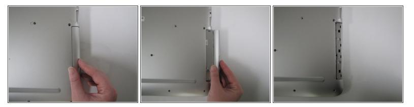
• On the right-hand corner of the laptop, remove the CD-ROM by pressing the small button on the side. Pull it out of the laptop, and set it to the side.
