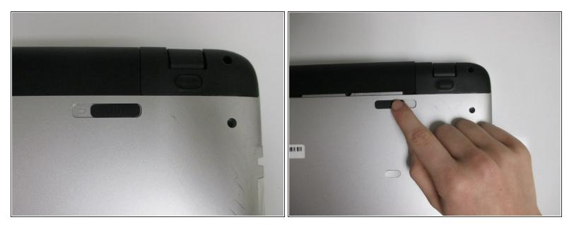
• Slide the bar with the battery icon, on the right of your laptop, to the left to release the battery.
