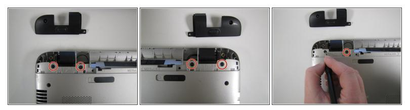
• Remove the four 6.5mm Phillips #00 screws that were underneath the black corner covers.
