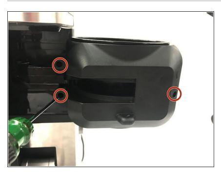
Remove three 6mm screws with Phillips head screw driver.
