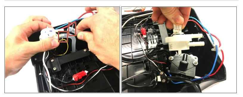
Detach valve tubes from valve by squeezing pins and pull tubes away from valve
