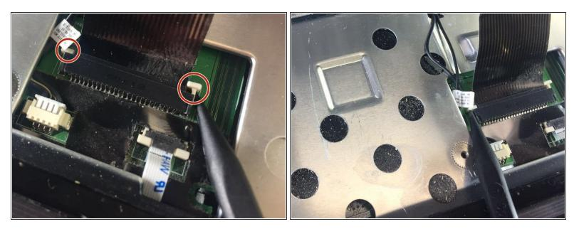
Use your plastic spudger to unlock the two white sliding connectors located on the left and right side of the device by gently pushing them out.
