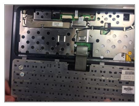
• Flip the keyboard over. It may be easiest to hold it up in order to detach its wire assembly.
