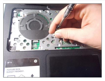
Remove the five 3 mm PH1 Phillips head screws underneath keyboard.
