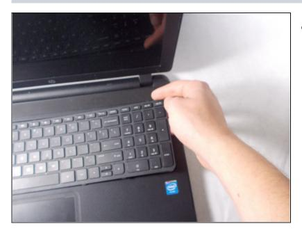
Pry up and detach the keyboard. Starting at the top, slowly work the side and pull the keyboard away from you to unseat the bottom tabs.
