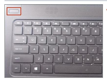
Turn power off using the power button located in the top left corner of the keyboard. Press and hold the power button for 3 seconds until it turns off.
