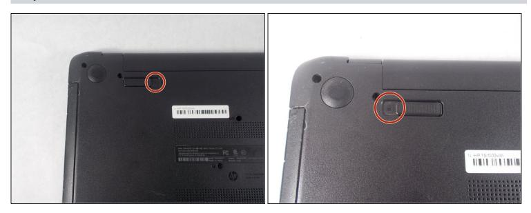
Slide the left switch to the right so that the icon of a locked padlock is no longer visible and the icon of an unlocked padlock is now visible.
