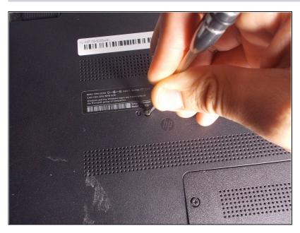
• Remove the thirteen 7 mm PH1 Phillips head screws from the bottom of the laptop.
