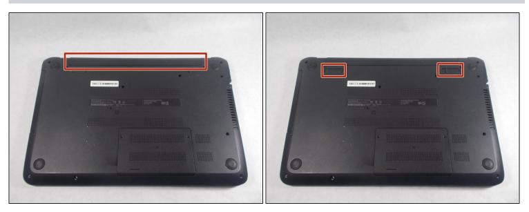
• Locate the battery and the two switches that release the battery when they are unlocked.
