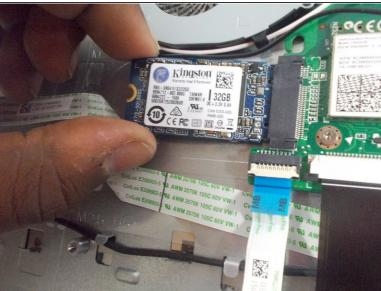
Grab the top and bottom edges of the SSD and carefully pull it out from the motherboard.
