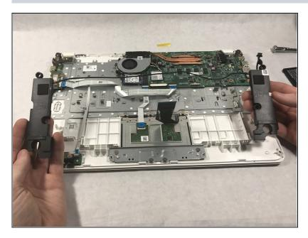
Simply lift upwards on both speakers, and they will remove from their position.
