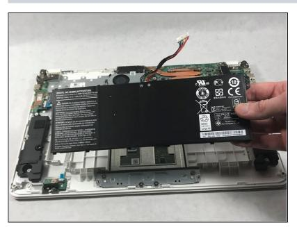
Gently lift the battery out and remove it from the laptop casing.
