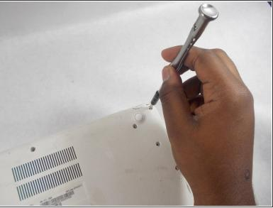
Unscrew the eighteen 6 mm PH0 Phillips head screws from the back of the device.
