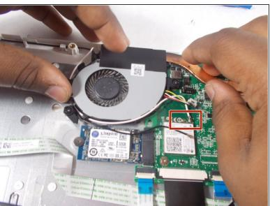
Carefully unwrap the black and white wires from around the fan cover.
