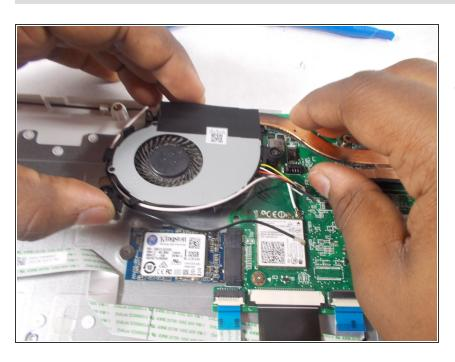
Grab the fan by its cover and the brass colored piece of metal and carefully lift up and pull out the fan from the device. To reassemble your device, follow these instructions in reverse order.
