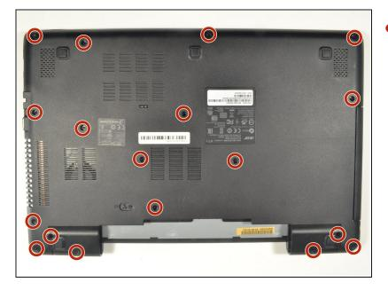
Using a #0 Phillips screwdriver, remove a total of eighteen identical 8mm Phillips screws and set them aside.
