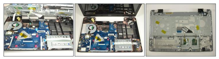
• Once all three ribbon cables are disconnected, lift off the top cover with the keyboard and touchpad.
