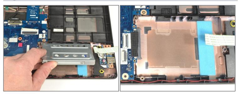
• Lift up the hard drive carriage on the edge closest to your body to remove it.
