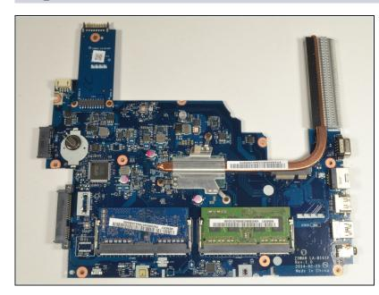
• Lift the motherboard out of the case.
