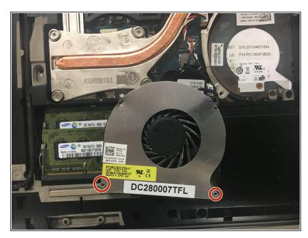
Unscrew the 1mm screws on the fan case.
