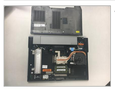
Remove the back cover by sliding it downwards.
