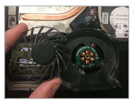
Remove the fan by pulling it away from the motor.
