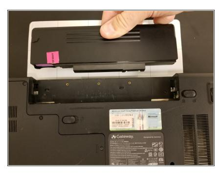
• Pull the battery pack out of its slot.
