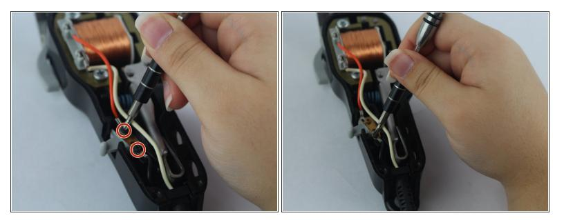
Unscrew the two black 5.556 mm Phillip head screw on the power switch with a Phillips #0 Screwdriver.
