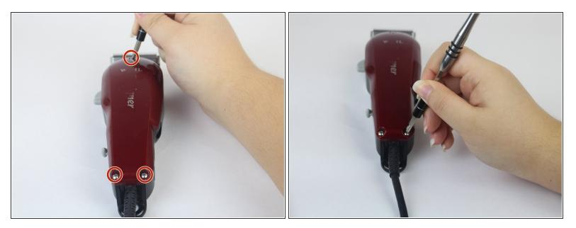
Unscrew the 12 mm Phillips head screws located at the top of the cover and at the bottom two corners, using a Phillips #1 Screwdriver.
