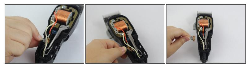
• Shimmy the power switch off the mount until it is completely removed.
