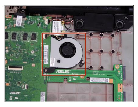
The fan is located near the upper left hand corner of the device, connected to the motherboard and right beneath the wireless card.
