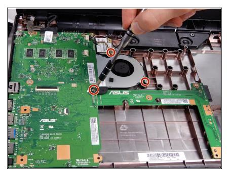
Using the J00 screw bit in the iFixit tool kit, remove the three screws securing the fan to the case. One screw connected to the bottom case (4cm), one connected to the motherboard (4cm), and one screw connected to the Wireless Card (5cm).
