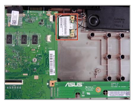
• The wireless cared is located in the upper left portion of the device case, right above the fan and attached to the motherboard.
