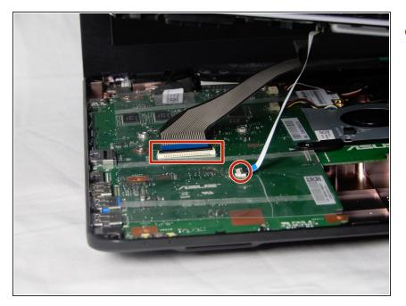
Observe where the ribbons connect to the motherboard, there are two connections. Each connection has a black clamp. To remove the ribbon, lift the black clamp up to disconnect it.
