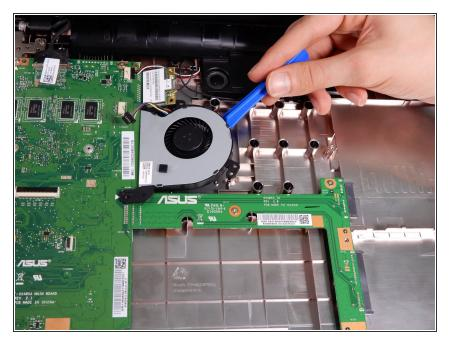
• Carefully remove the fan from the case using the blue iFixit opening tool.
