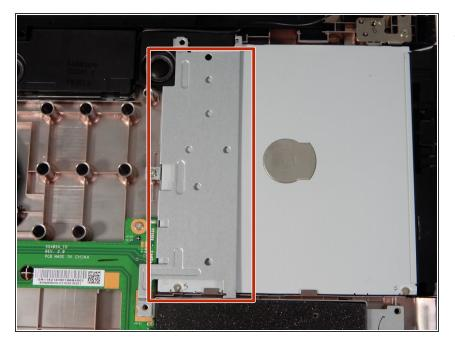
• After removing the seven screws, lift the metal fastener from the disc drive with the plastic opening tool.
