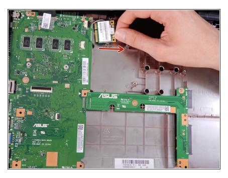
• Carefully slide the wireless card to the right, and remove it from the device.
