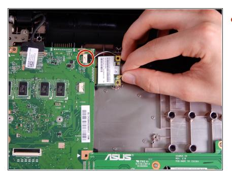
There is only one cable connecting the wireless card to the antenna.
