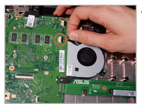
There is a bundle of wires connecting the fan to the motherboard. Disconnect them.
