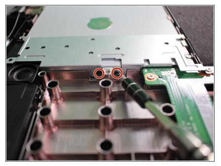
• Use the Phillips #00 screwdriver to remove the two screws (2.7 mm) on the side of the disc drive fastener.
