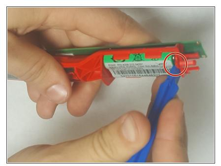
Pry away the battery using an opening tool from the battery housing. This will break the circuit and avoid electric shock.
