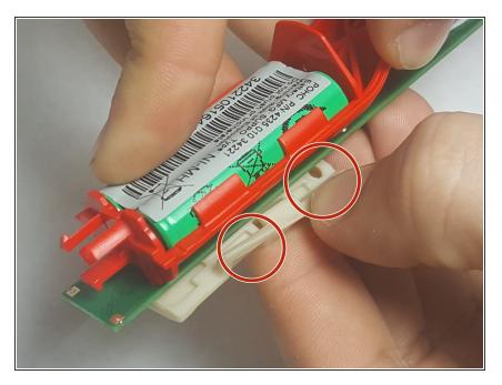
Remove the white circuit board cover as shown. This cover will require you to pry off the piece from the groves.
