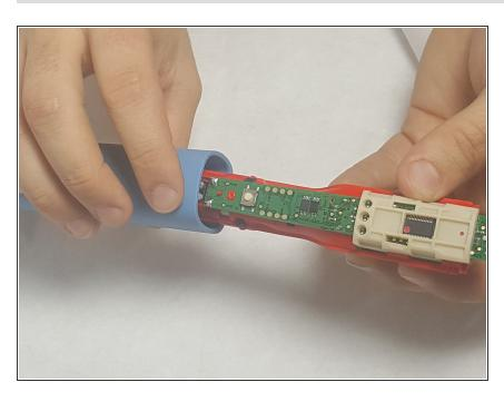
Next you will be able to remove the internal electronic mechanism as shown in the figure.
