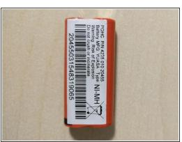
Well, the VOLTAGE of this battery is about 2.8 to 2.9 Volts. The size is same as that of TWO AAA Cells. Two AAA in series can easily replace the existing battery. Ni-Mh AAA cells of Energizer can do the job. Disconnect the existing battery but don't remove the metallic connection to the circuit.
