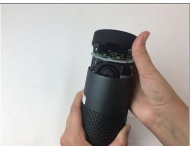
Pry up and remove the soft plastic casing from the rest of the device.
