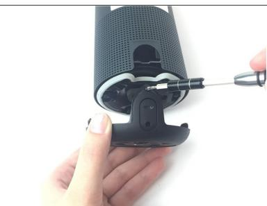
Remove the screw that is above the charging port.
