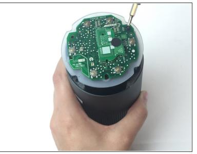
Remove the 3 screws holding down the top circuit board.
