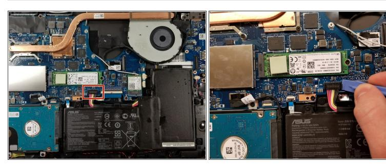
Wedge an opening tool under the battery's bundled cable connector, and gently pry the connector up and to disconnect the battery.
