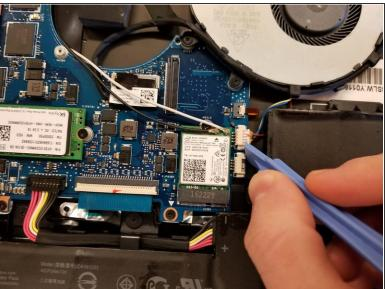
Using the iFixit opening tool, gently pry the CPU fan connector out of the socket.
