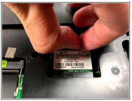
Disconnect both the black and white coaxial connectors from the WiFi card by pulling up on the gold colored piece.
