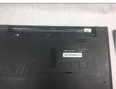
Rotate the battery up and remove it.
