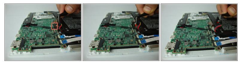
Carefully disconnect the battery cable from its connector on the mainboard.
