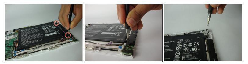
To unscrew the first speaker, use the Phillips #0 screwdriver to unscrew the 2 screws- head
