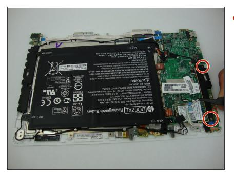
For the second speaker, repeat the previous step by unscrewing the two screws.
