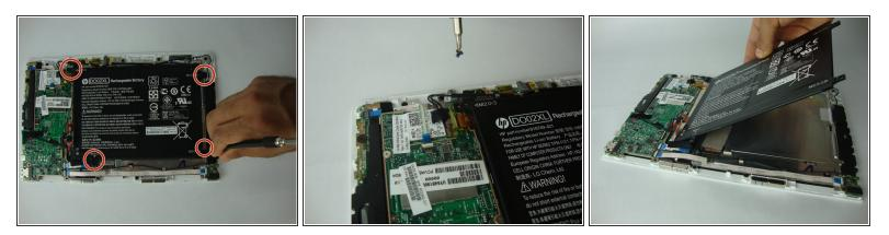
• Using the Phillips #0 screwdriver, carefully remove the 4 corner screws that hold the battery to the display panel.
