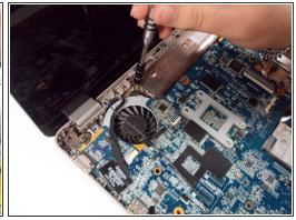
Remove the two motherboard screws and the fan screw that holds it on the the rest of the computer with a Phillips #1 screwdriver.
