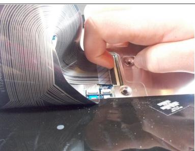
Pull up the latch that connects the keyboard connector the the motherboard.
