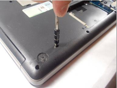
Remove four Phillips PM2.5x3 screws in the battery bay, and remove ten Phillips PM2.5x6.5 screws on the base enclosure with a Phillips #1 screwdriver.
