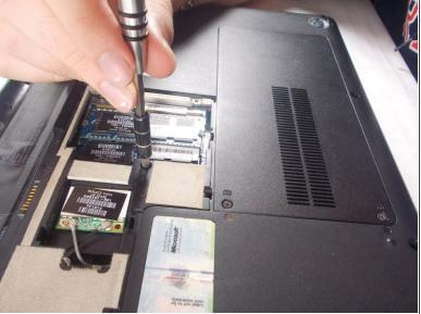
Unscrew the final Phillips 2.5x5 keyboard screw with a Phillips #1 screwdriver.
