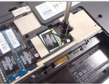
Remove the Phillips PM2.0×3.0 screw that secures the WLAN module to the computer with a Phillips #0 screwdriver.
