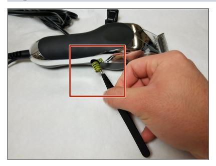
• Remove the spring on the side of the body using <u>tweezers</u>.
