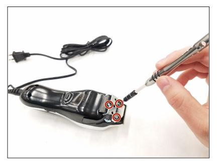
Remove the three 9.0 mm JIS #1 screws attaching the base of the blade assembly to the body.
