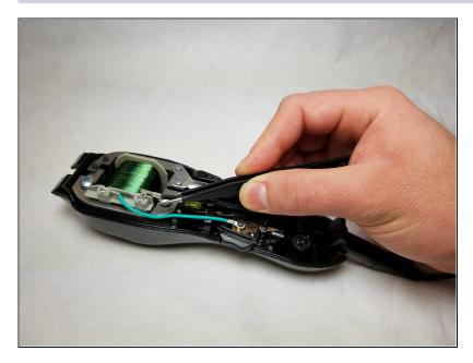
• Unplug the cord terminal from the motor connector.
