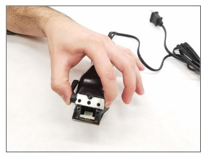
• Lift the base of blade assembly straight up off of the body.
