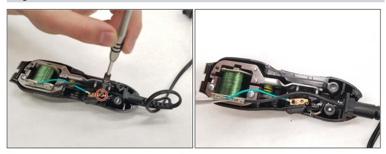
• Remove one 7.5 mm JIS #1 screw from the switch base.
