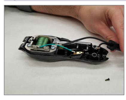
• Remove the cord from the device base by pulling gently.
