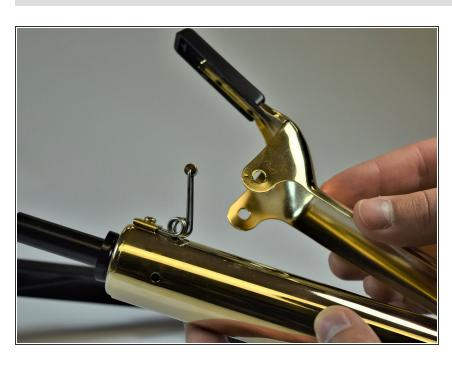
Once both screws have been removed, continue to remove the top clamping half of the mechanism from the body of the Iron.
