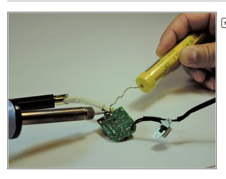
To reattach the new temperature control switch, solder the piece onto the board.
