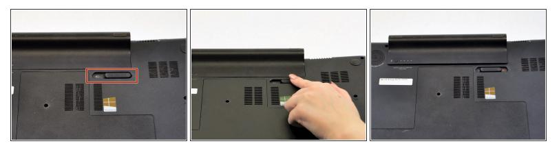
• Slide the battery release latch to the left which is located on the right-hand side of the battery.
