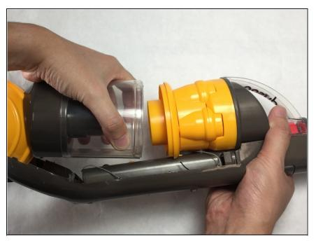
Separate the bead cylinder and the fan compartment by pulling the bead cylinder away from the fan compartment.
