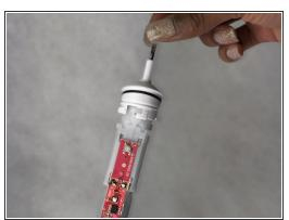
Using the pliers, rotate the head base 90 degrees counterclockwise and remove core from the handle.
