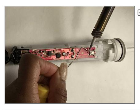
Attach the new button by soldering the 4 terminals with new solder.
