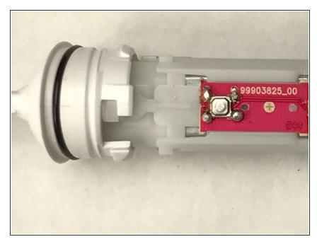
Locate the 4 terminals connecting the power button to the circuit board.
