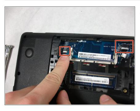
Unplug the two exposed cables from the motherboard.
