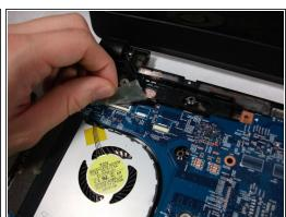
Unplug the ribbon cable connected to the USB Hub, the network card, and the monitor cable.
