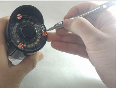
To remove the motor, you must begin by removing the three screw caps and the 15mm JIS 0 screws associated with them located on the plastic containment shell that the camera is in.
