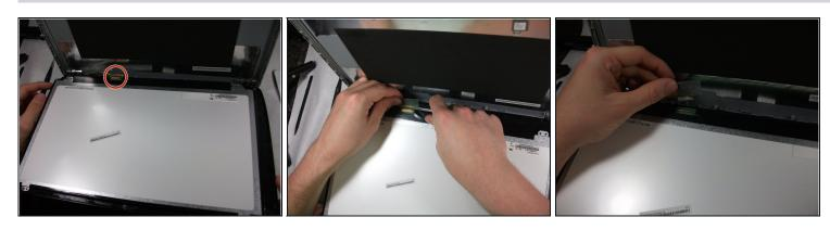
• Peel up the tape over the connector and unplug the screen from the laptop.
