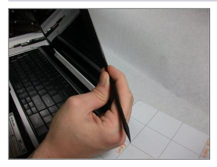
Take the plastic spudger and pull up the tabs on all four sides of the screen molding.
