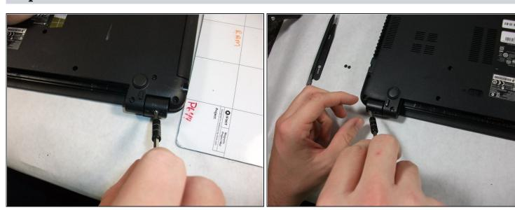
Unscrew both of the 3mm Phillips 01 screws on both hinges using the matching screwdriver.
