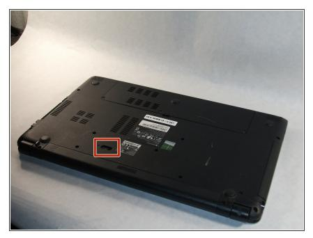
Make sure the laptop is turned off and flipped over so that the bottom is facing up. Then, locate the battery clip as shown.
