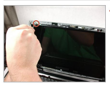
Unscrew the four 3mm inch Phillips01 screws on the screen bracket.
