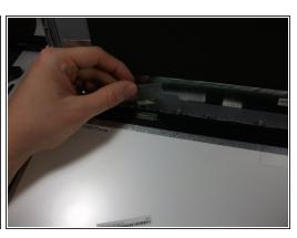
Peel up the tape over the connector and unplug the screen from the laptop.
