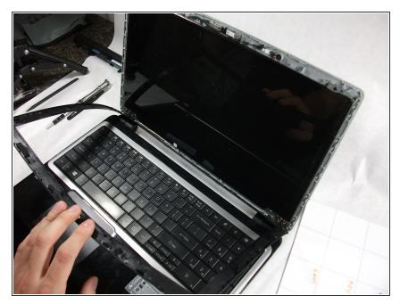
Carefully remove the screen molding. Be aware that the screen molding will not come out all the way.
