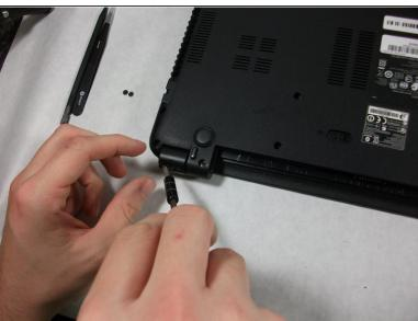
Unscrew both of the 3mm Phillips 01 screws on both hinges using the matching screwdriver.
