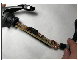
Pry off the housing using a plastic spudger.
