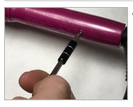
Remove the Philips #1 22 mm screws.
