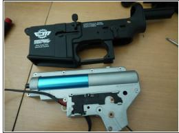
Set the selector switch to the semi-auto position, and remove the gearbox from the lower receiver, pulling it upwards and slightly forward.
