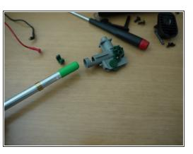
You can disassemble the inner barrel and hop-up unit by adjusting the hop-up to its lowest setting (turn the knob counterclockwise until it stops), removing the small green clip on the underside of the hop-up unit, then pulling the barrel out. You can also remove the hop-up bucking as well as a small brass ring that helps support the barrel.
