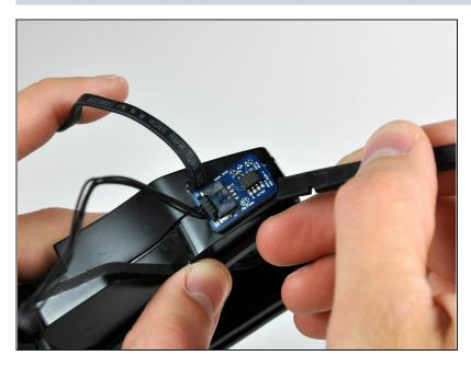
Use the flat end of a spudger to pry the ambient temperature sensor off the adhesive securing it to the left speaker.
