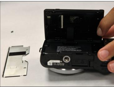
• Using the plastic opening tool, remove the larger backplate from the LCD screen.
