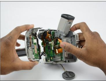
• Now that all of the screws are removed, gently pull off the side panel of the camcorder.
