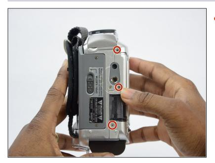
• Remove all 3.75 mm screws from the bottom of the camcorder.
